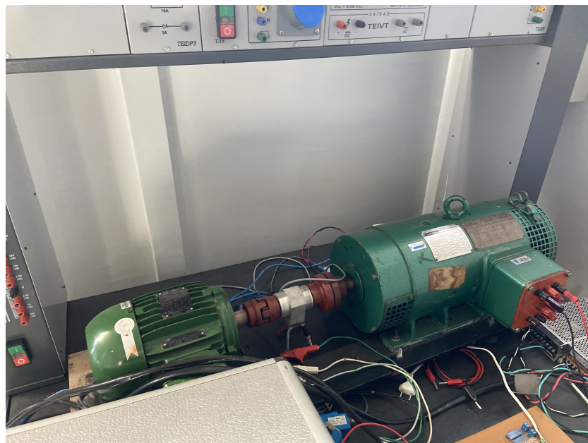
Figure 3.9: Motor and CC generator with coupled shafts employed in the experimental tests
