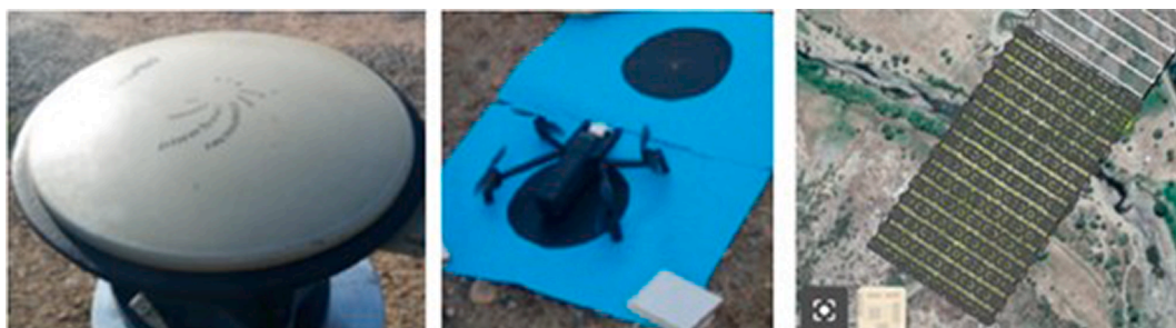
Fig. 8. Details of the aerial survey of the topography on the bridge over the Pianco River.
