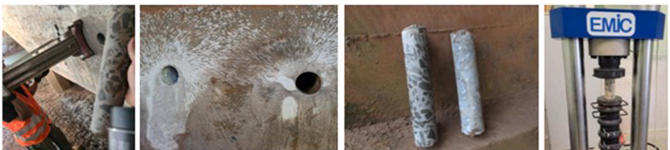
Fig. 20. Extraction of specimens to determine compressive strength.
