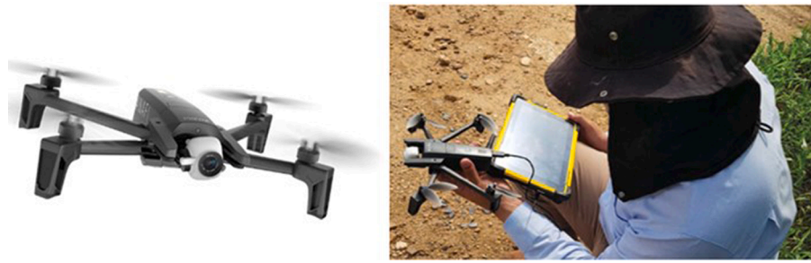
Fig. 9. Using the Parrot ANAFI UAV in the photogrammetry with 180° camera gimbal.
