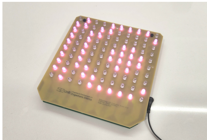
Figure 3.19: LED Board designed for the phase distribution matrix mapping.
