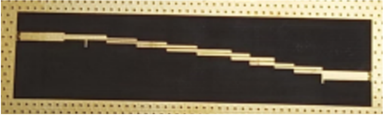
Figure 4.13 – Order 8 Parallel Couple filter with input and output stub for impedance matching. Source: Own elaboration.
