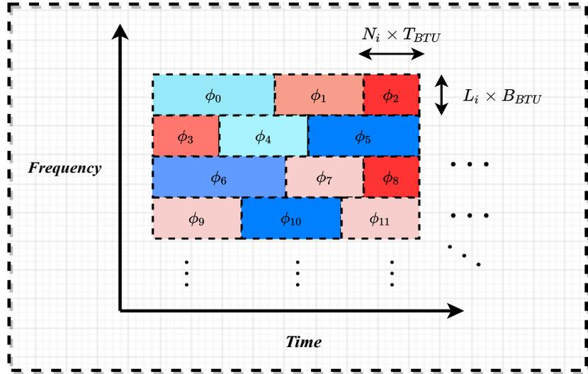
Figure 12 – Distribution of BTU resources  $\phi_i$  in a DVB-RCS2 SF. All  $\phi_i$  occupies the same bandwidth in an SF.
