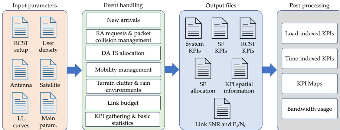
Figure 8 – General structure of the system-level simulator, with examples of input and output files. The event handling subsystem is responsible for RCSTs transmission management.
