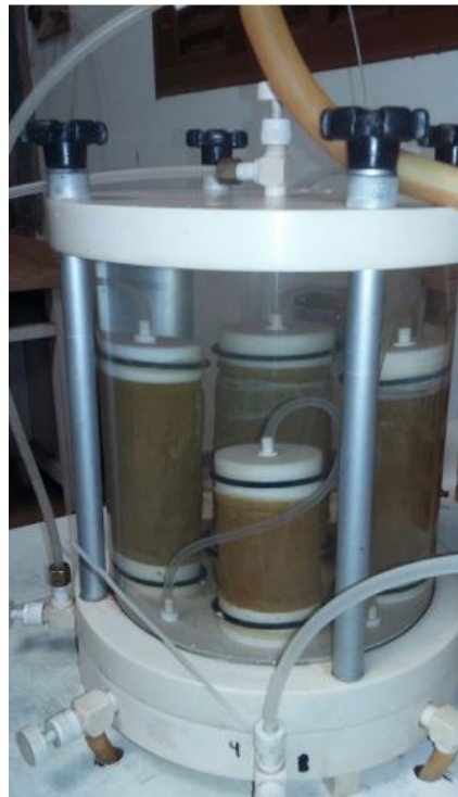
Figure 7. Detail of the soil cylinders (columns) with heights of 6 cm and 12 cm.
