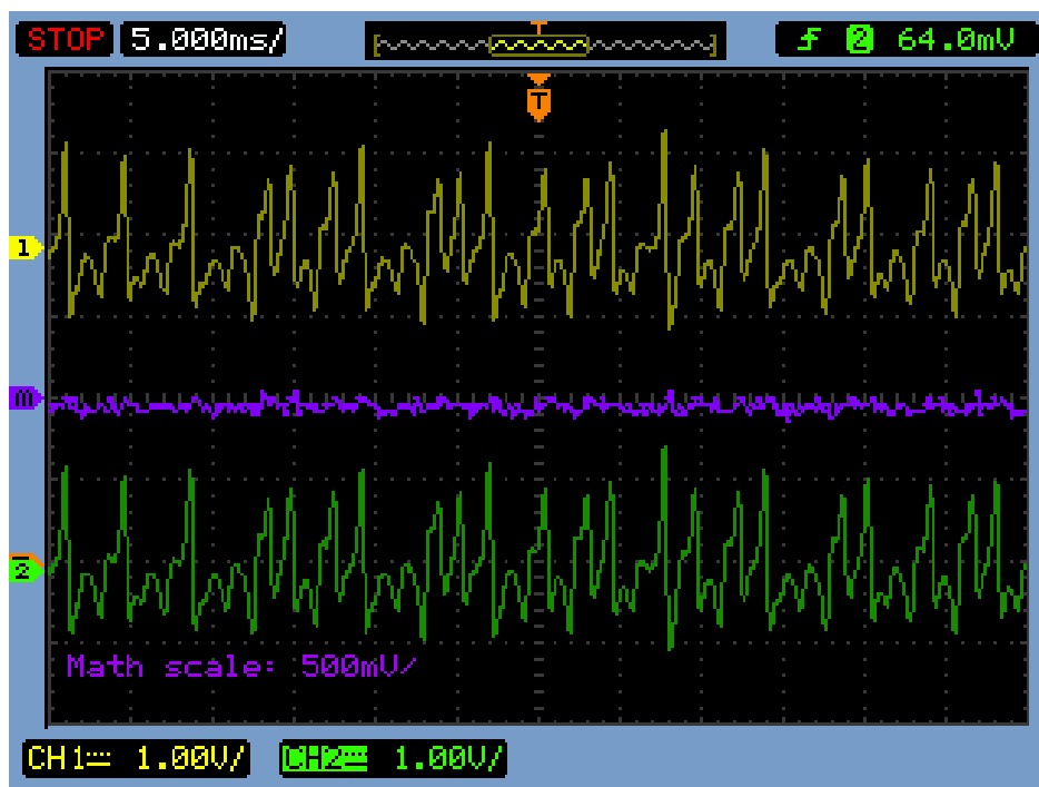
Figure 5.22 – Observation of experimental y_m(t) (Channel 2), y_s(t) (Channel 1), and e_y(t) (MATH).
