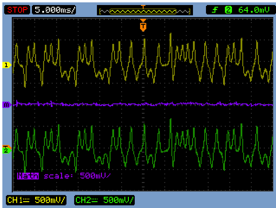
Figure 5.21 – Observation of experimental x_m(t) (Channel 2), x_s(t) (Channel 1), and e_x(t) (MATH).
