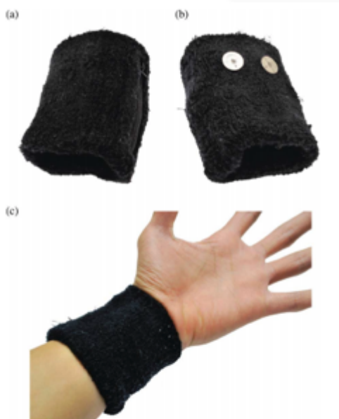
Fig. 3. Wearable EDA sensor. (a) Final packaging in an attractive and inconspicuous wristband. (b) Disposable Ag/AgCl electrodes attached to the underside of the wristband. (c) Wearable EDA sensor can be worn comfortably on the wrist for long periods of time and during daily activities.
