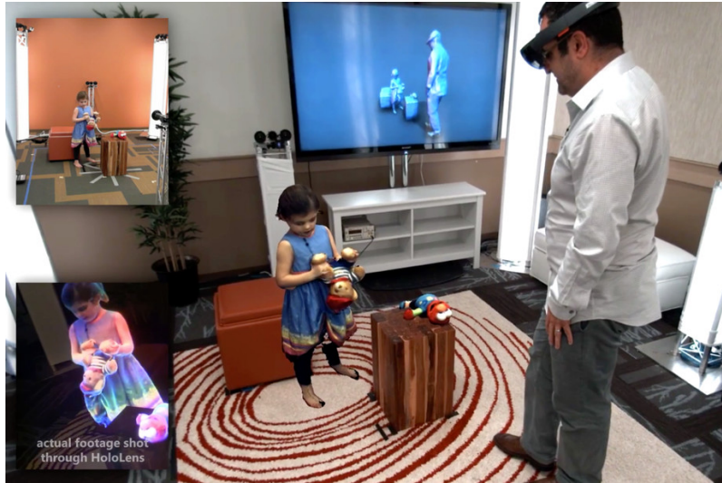
Figure 2.18: Demonstration by Microsoft of a user viewing a remote located kid through a MR device. Top left shows the real scene and bottom left the way the scene is viewed in the Microsoft's MR HMD, called HoloLens.
