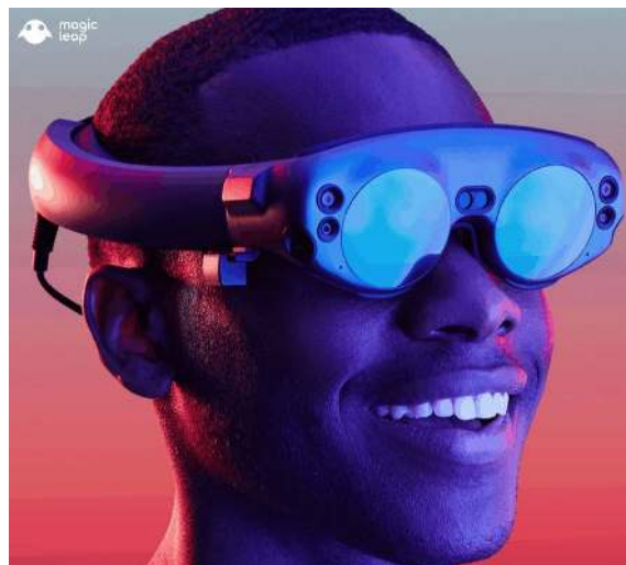
Figure 2.19: Magic Leap One mixed reality head-mounted device. In the image it's possible to see some of the many sensors the device has, including depth sensor.
