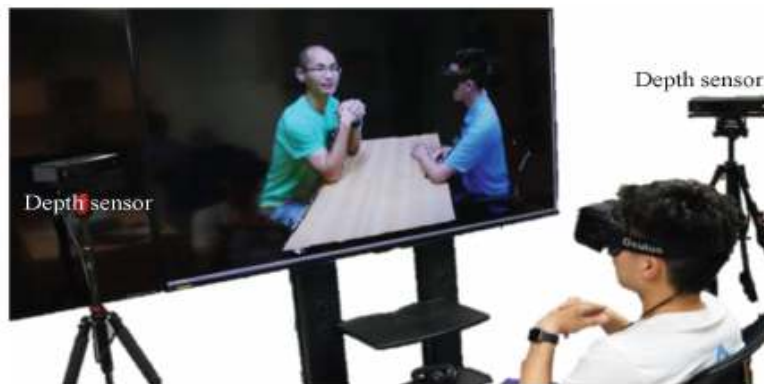
Figure 2.17: User with a Oculus Rift VR glass interacting with another user, while being captured by a setup of three (one hidden) RGB-D Microsoft Kinect sensors. A synthesized scene with the two users is shown in the TV in the back.
