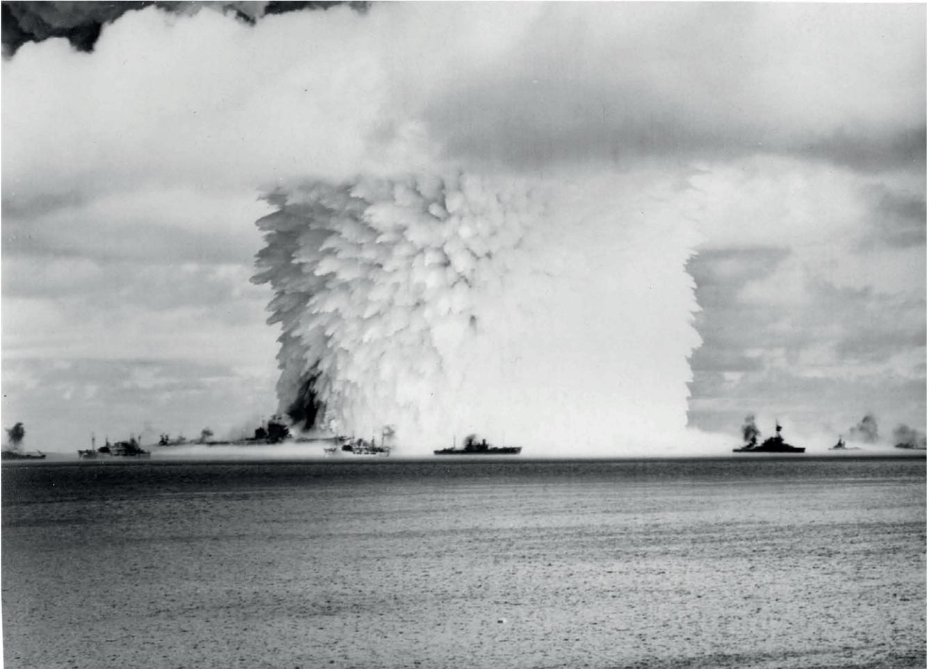
**FIGURE 22 - VIEW FROM ENYU 10 SECONDS AFTER EXPLOSION SHOWING STERN OF SARATOGA RISING 43 FEET ON FIRST WAVE CREST. NOTE THAT STACK APPEARS UNDAMAGED.**
