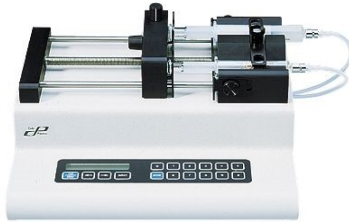
Figure 6.3 – Syringe pump from Cole & Parmer , model KDS 101.
