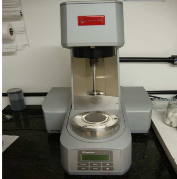
Figure 6.7 – Rheometer Physica MCR 301 from Anton Paar .
