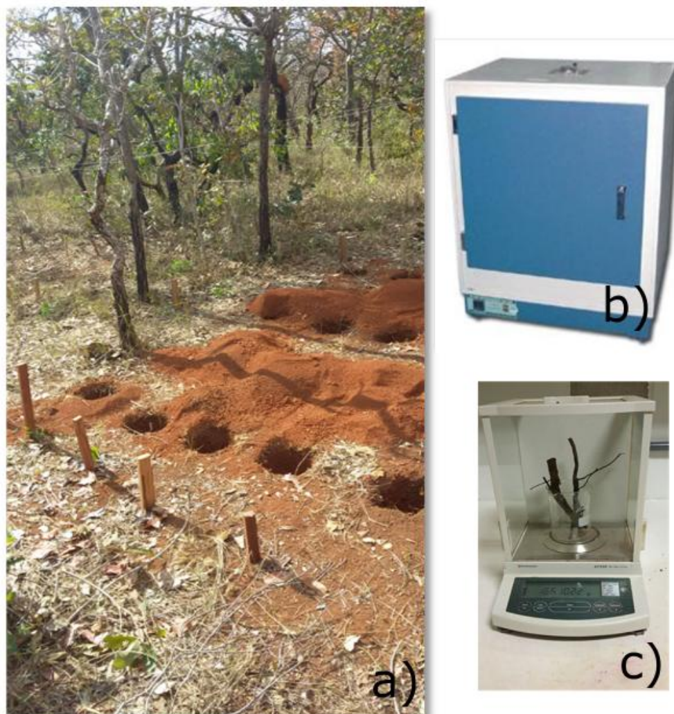
Figure 3.3 – a) Crops of biomass samples collected; b) stove model 032/1 from MARCONI; c) Analytical balance model Shimadzu Ay220.
