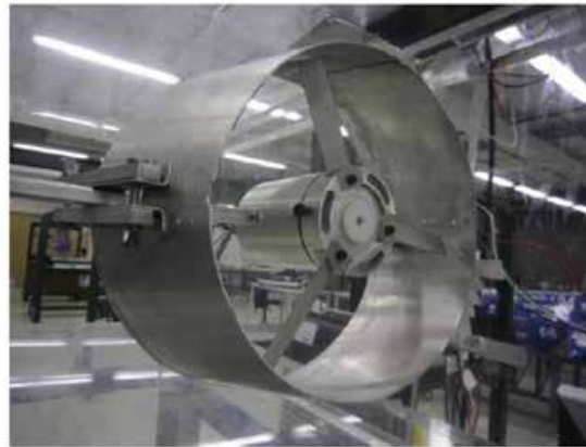
Figure 7.9 – Conical diffuser-augmented turbine by Kosasih and Saleh [83].
