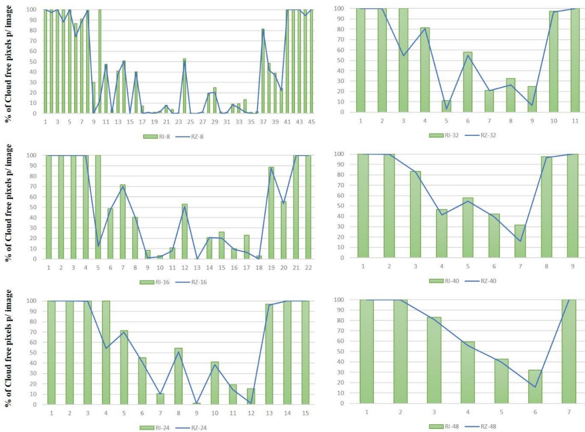
Figure 3.6. Comparison between compositions with regular intervals (with and without the use of zenith sensor angle restriction) considering the percentage of valid pixels in the composition.
