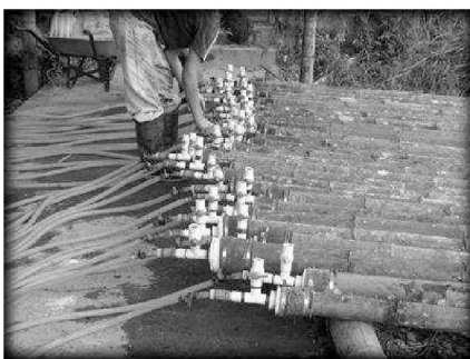
Figura 7: Método boucherie (Fonte: www.bamboocostarica.com/Immunization.html ).
