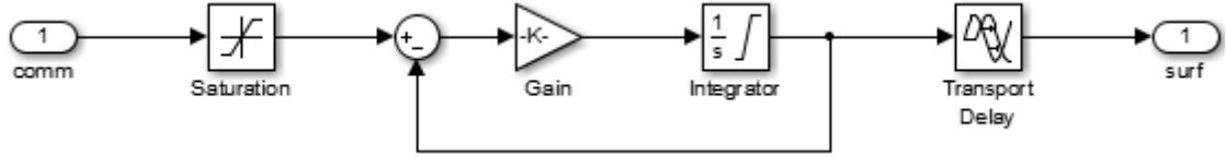
Figure A.1: Actuator dynamic model in Simulink. Gain K = 1/\tau_a (control surfaces) or 1/\tau_T (engine). The Transport Delay block inserts a t_{d,a} or t_{d,T} delay.
