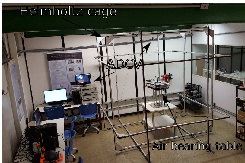
Figure 2.1: Nanosatellite simulator into the Laboratory of Aerospace Science and Innovation (LAICA/UnB).
