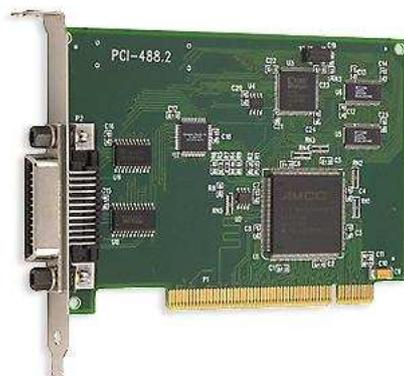
Figura 2.3 - Interface PCI-GPIB.
