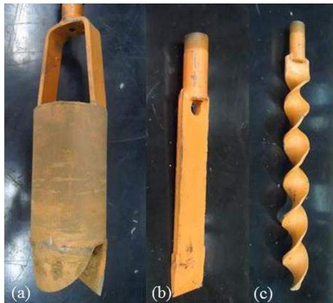
Figura 2.9 – (a) Trado concha (b) Trépano (c) Trado hélice.
