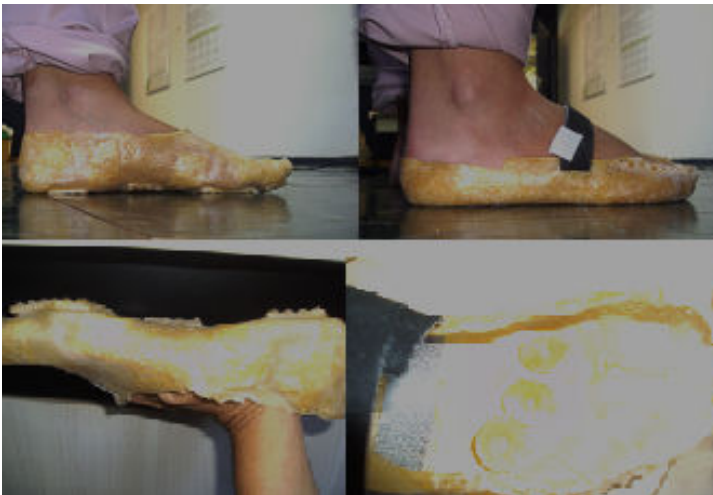
Figure 6. Photo of the shock-absorbing insole prototype with the shock-absorbers highlighted.
