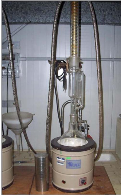
Figura 5.9 – Extrator Soxhlet.
