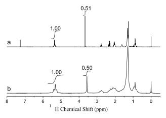
**Figure 1.** <sup>1</sup>H NMR spectra of a standard sample with 50% of FAME; (a) 7.05 T spectrometer; (b) 1.40 T spectrometer.
