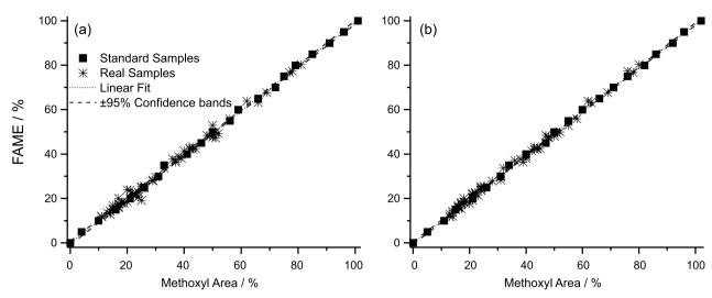
Figure 2. Calibration curve obtained with standard samples and known concentrations, and predicted FAME concentration of real samples. Integrated intensities obtained from: (a) 7.05 T spectrometer, with  $R^2 = 0.9991$ , RMSEP = 1.0332; (b) 1.40 T spectrometer, with  $R^2 = 0.9995$ , RMSEP = 1.2401.
