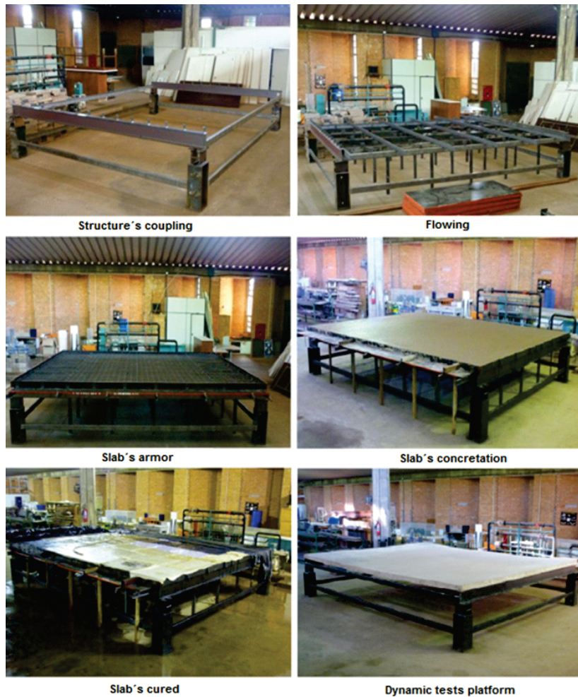
Figure 8 – Different steps of constructing the dynamic tests platform
