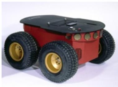
**Figura 3.1.** Plataforma experimental Pioneer 3-AT
