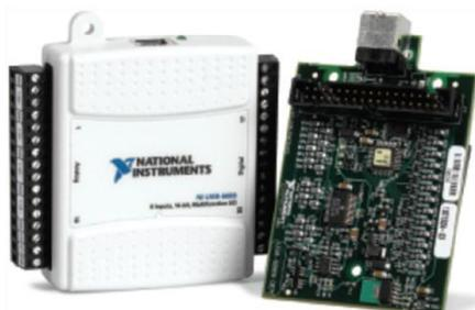
Figura 4.20 – Placa NI USB-6009 (NATIONAL INSTRUMENTS, 2010)
