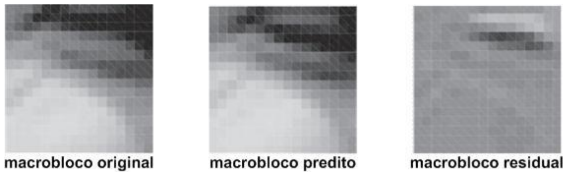
Figura 2.7: Macrobloco residual = Macrobloco original – Macrobloco predito.
