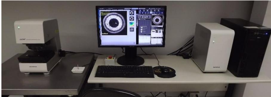
Figure 4.21 Confocal laser microscope.
