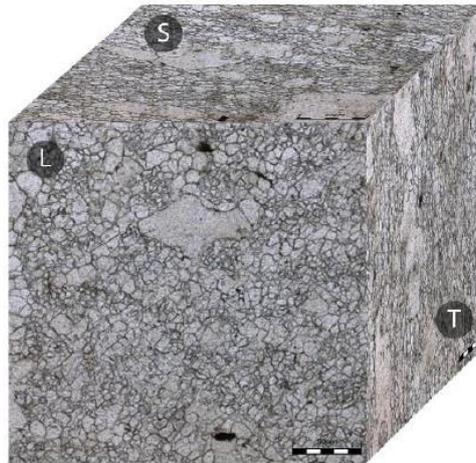
Figure 4.1. Microstructure of the Al7050 [71].
