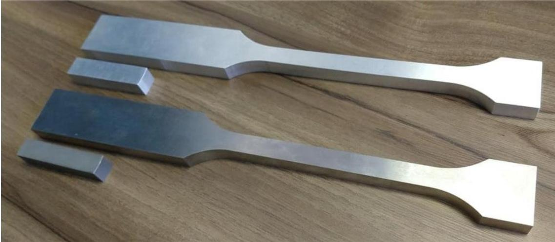
Figure 4.6. photograph of pad/specimen made of 7050 T7451 aluminum alloy on the top and ASTM 743 CA6NM steel on the bottom.
