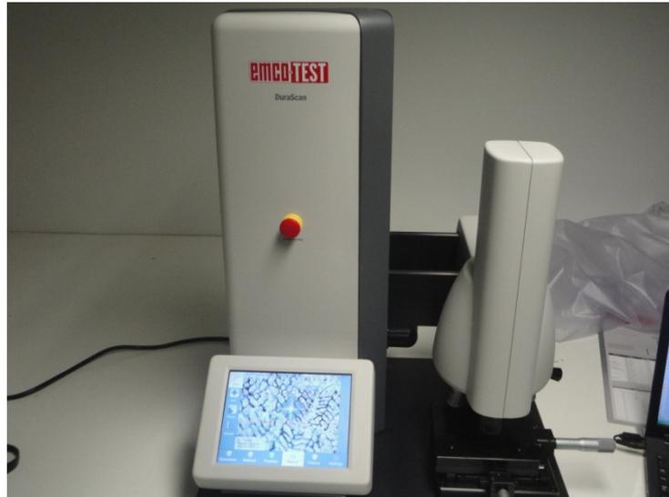
**Figura 3.10:** Durômetro Emco-Test.
