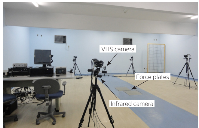
Figure 1. Panoramic view of the UEG Laboratory, indicating force plates, infrared cameras and VHS cameras
