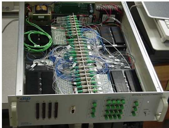
Figura A.4 - *Optical cross-connect* (OXC) da rede OMEGA.
